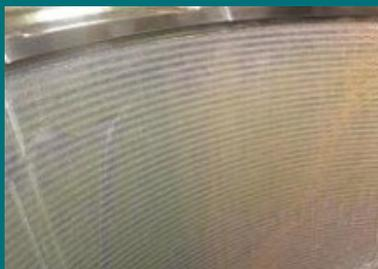
Figure 7. new Cylinder liner
