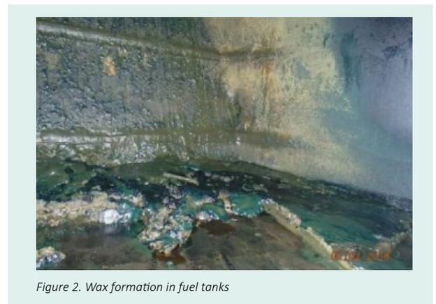
*Figure 2. Wax formation in fuel tanks*
