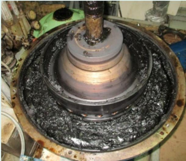
Figure 11. Purifier every 3 hours after loading VLSFO
