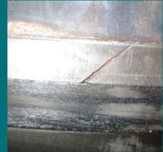
Figure 6. Deposits behind piston rings
