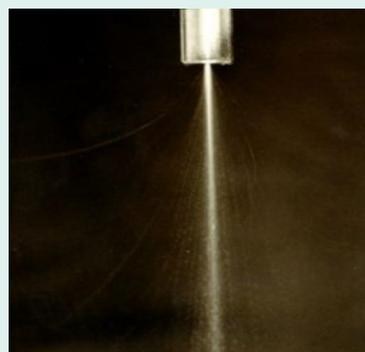
Figure 9. spray pattern after 100 hours using stressed fuel
