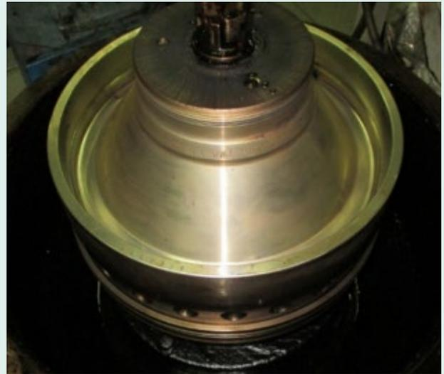
Figure 12. Same purifier, same fuel, 24 hours after additive application
