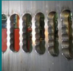
Figure 4. Scavenge ports after switch to VLSFO
