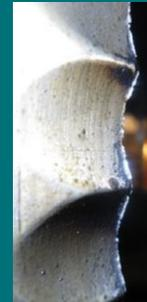
Figure 5. Burr on liner surface
