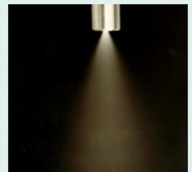
Figure 10. spray pattern after additive application to same fuel
