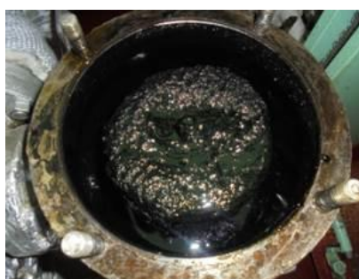
High pour point solids in fuel lines, blocking fuel systems and causing fuel starvation
