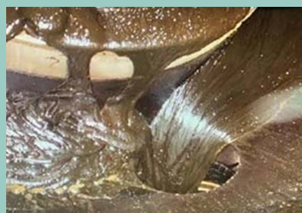
Wax n-paraffin wax crystals separating in fuel due to lower temperatures
