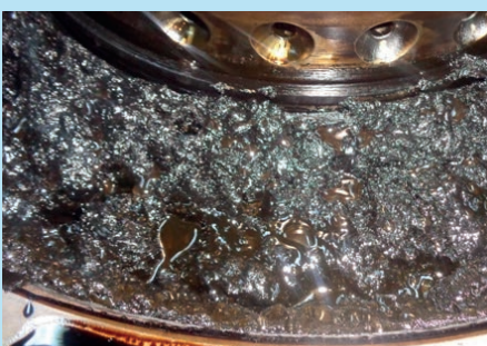
Distillate Distillate aging, polymerisation and fuel instability
