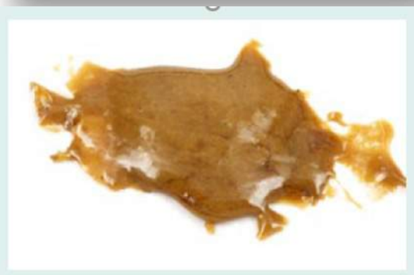
Gums: Sticky oxidation product (Adherent insoluble). Become impregnated with inorganics (metals, cat fines etc.) and act like a grinding paste on surfaces.
